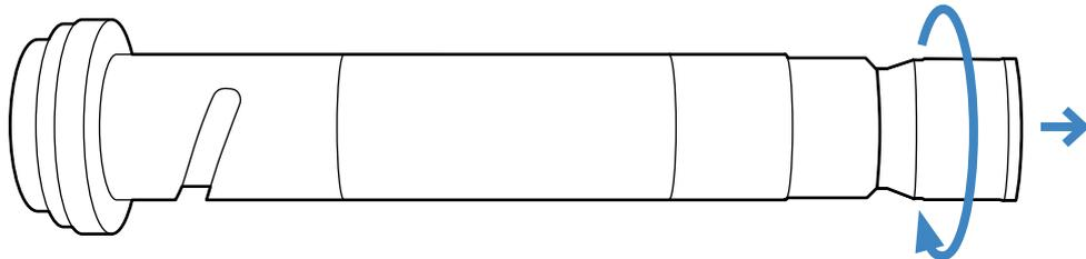
**1** Unscrew the optical tip of the probe to remove it
